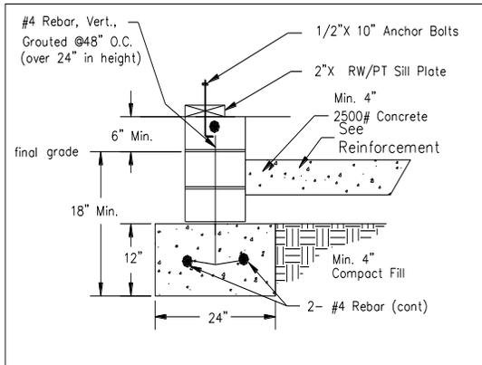
Figure 9. Slab construction stem wall
